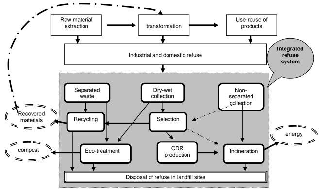
Figure 3: Integrated waste system with activities from the manufacturing, consumption, recovery and disposal chain.
